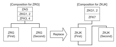
\*First analyzer: This analyzer is connected to  $O_2$  signal directly and indicate  $O_2$  indication. Second analyzer: This analyzer is connected to  $O_2$  instantaneous value from first analyzer and could not indicate  $O_2$  indication.
